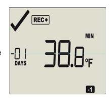
The logger will store and display 30 days of min/max temperatures.
